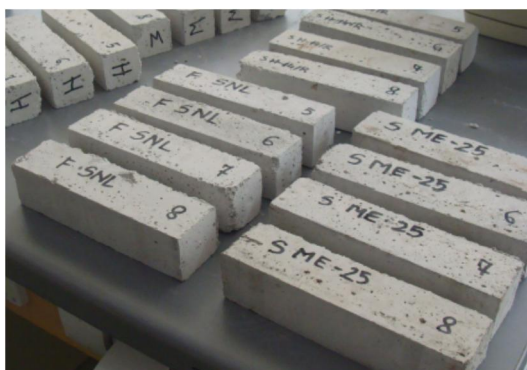
Fig. 2 Condition of the plaster samples after examination on resistance to salt crystallization
